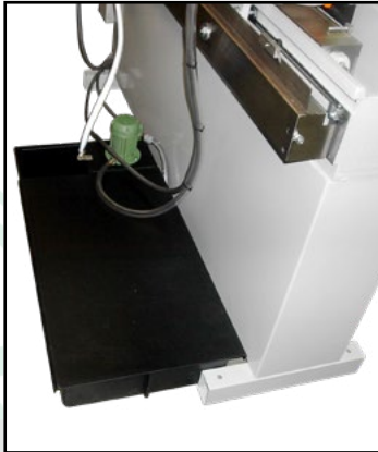
Vasca esterna External coolant tank with pump Внешняя ванна
